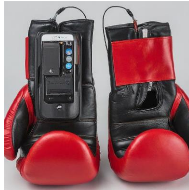
Figure 3.14 Smartphone sensor in the boxing glove
