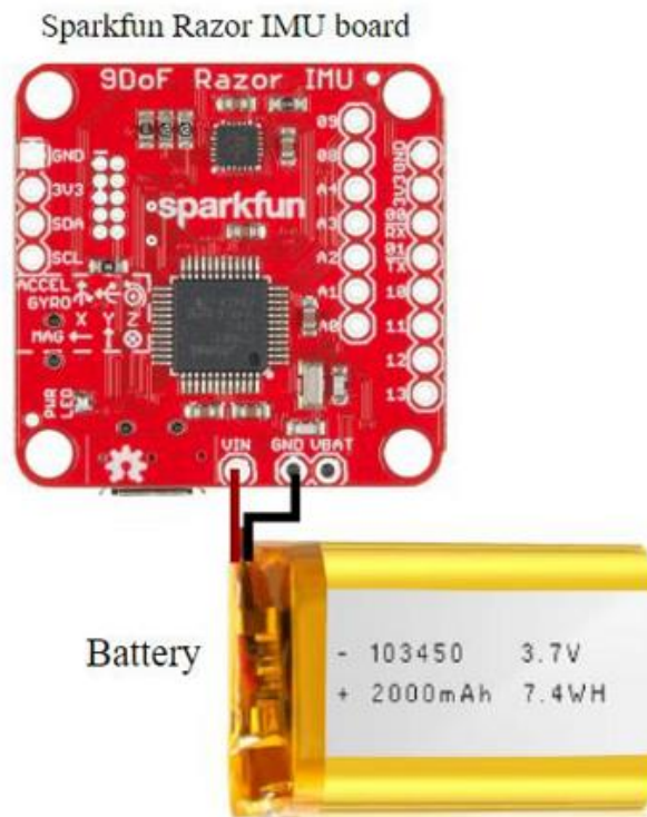
Figure 3.4 The wearable sensor including 9DOF IMU
